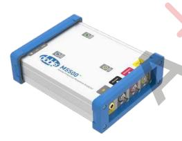
The M5500 Sweep Frequency Response Analyzer (SFRA) is the newest generation of SFRA diagnostic instrument from Doble. With incredibly fast sweep speed and expanded dynamic range, you can use the Doble M5500 test set to investigate the mechanical integrity of transformers, reactors and other equipment with windings. Coupled with the ease-of-use and powerful features of the new SFRA v6 Software, conducting SFRA testing and analysis of your apparatus has never been easier or more productive.
