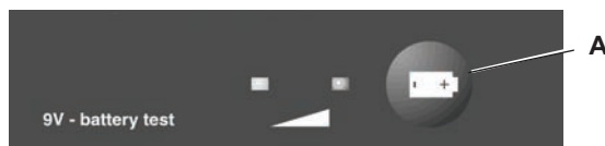
Figure 13: Battery Test Button
